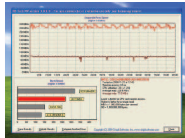
HD Tach (Intel SSD) – Note the very high read speeds and mediocre write speed
