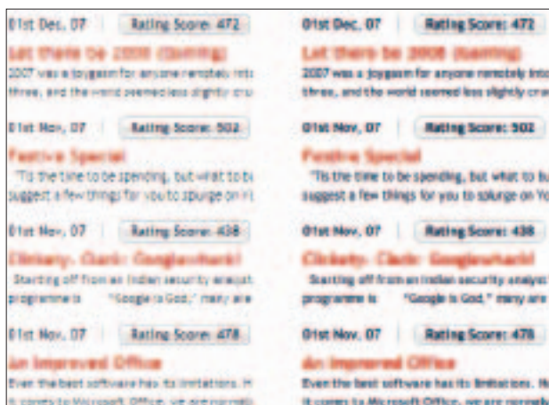
Left: text rasterised with GDI32.dll; right: rasterised with GDI++.dll
